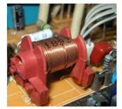
that can be easily magnetised; or in high frequency inductors, it will more likely to be just air.
