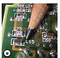
Surface Mount inductor in a Hard Disk Drive. Typical values can be 0.1nH – 220nH
