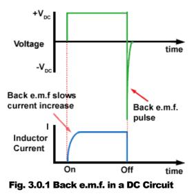
As the current through the inductor builds up, the rate of change of current has reduced, due to the back emf, and so has the back emf due to the reduced rate of change of the current. The electrical energy applied to the inductor has now been converted into magnetic energy and is stored in the magnetic field set up around the inductor.
