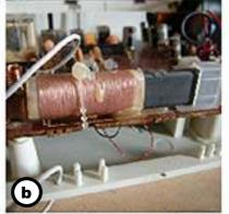
Ferrite rod antenna in an AM radio
