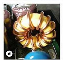
High current Toroidal Inductor in a power supply
